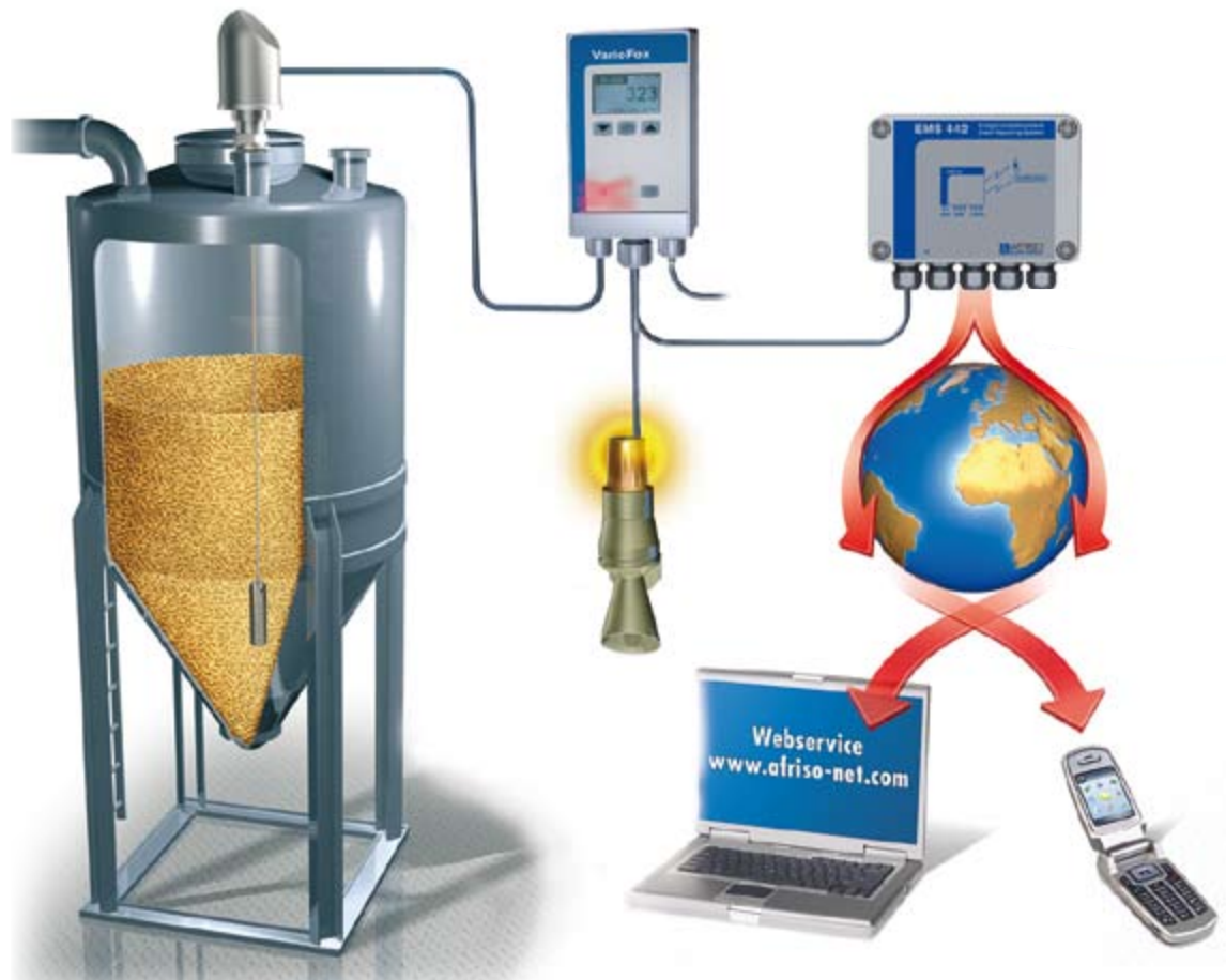
Measurement in a grain silo using PMG, VarioFox and EMS.
